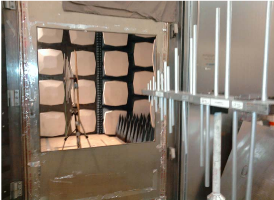
Figure 5. High Frequencies (100 - 200 MHz) Test Configuration Photograph
