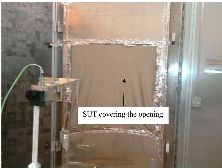
Figure 6. High Frequencies (above 1 GHz) Test Configuration Photograph
